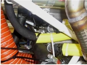
Secure all HILCOFLEX protective hoses against shift with tightening strips. Fix thermostat oil hoses to surrounding construction or to other hoses with tightening strips.
