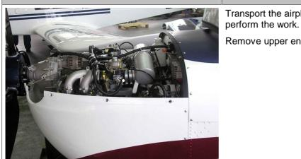
Remove upper engine cowling.
