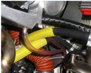
Remove original hose between oil tank and oil cooler, it will be replaced with E1 hose.
