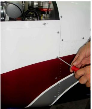
Set propeller (3-blade) upper blade vertically. Remove lower engine cowling. Unscrew upper bolts last. Helper unscrews upper screw on the opposite side and it will help during lower cowling removal. It is necessary to hold cowling during upper screws removal. Lower slightly cowling after upper screws removal and push cowling forward among propeller blades. Avoid contact cowling with nose wheel cover to prevent paint damage.
