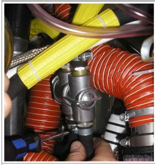
Check all thermostat oil hoses for flattening. Flattening is not permissible.
