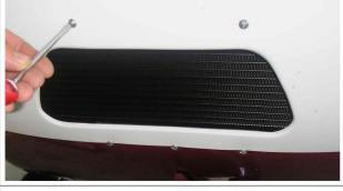
Install lower engine cowling, screw up water cooler.
