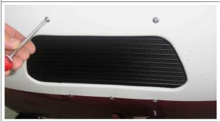
Remove 5 screws attaching water cooler to bottom engine cowling.
