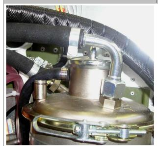
Slip hose clamp on the hose and put it on the oil tank elbow.
