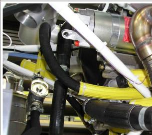
Train original hose from oil pump to E2 hose socket of the thermostat. Make smooth hose arch.
